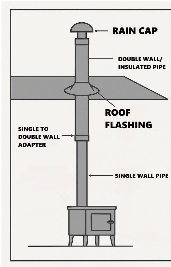
The simplified overview diagram above does not show items such as double wall pipe support bracket and double wall pipe joint clamps for securing double wall pipe joints (included) nor the stovepipe screws needed for install. Every installation is different. Verify pipe and stove distances from combustibles and use the proper type of pipes and parts as needed to maintain these clearances (mentioned below).
